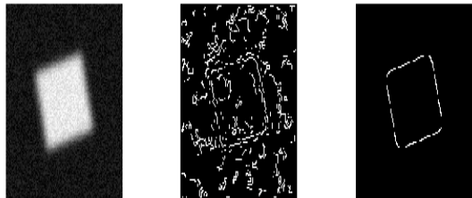
noisy image Canny filter, \sigma = 1 Canny filter, \sigma = 3
